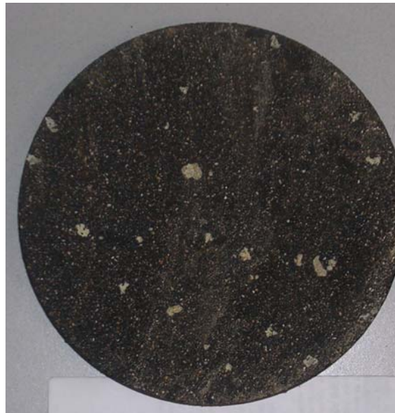
Figure 6. Type 3 Prills in AAD-Gravel Matrix.
