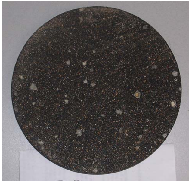
Figure 5. Type 2 Prills in AAD-Gravel Matrix.
